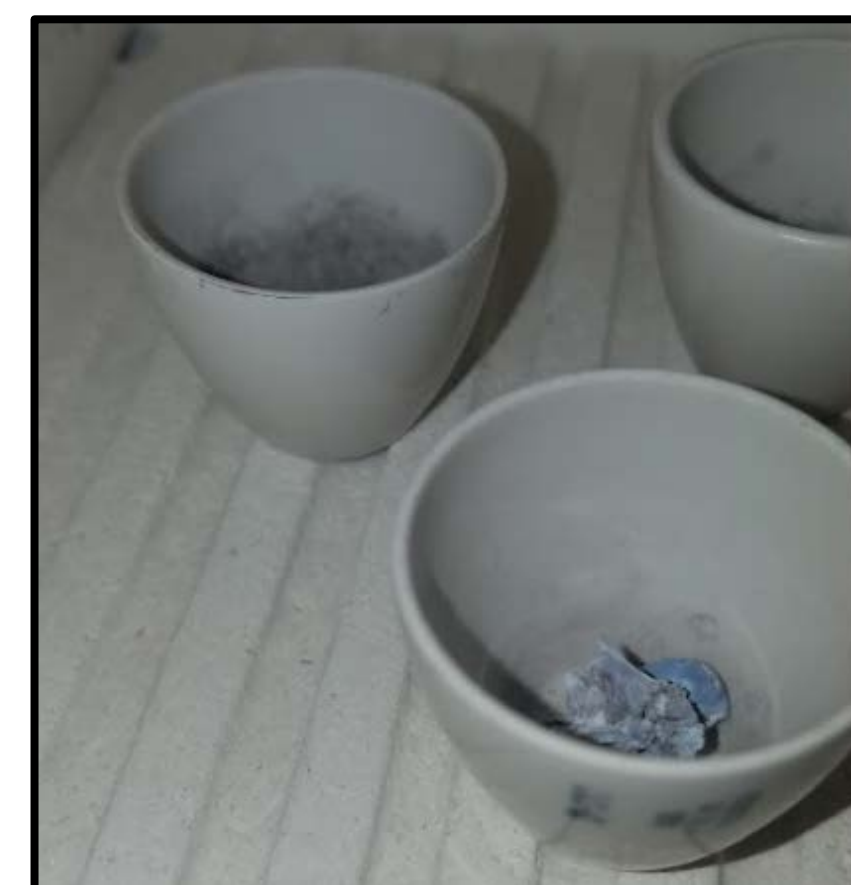
Figure 2. Armor tiles will be ashed in muffle furnace
